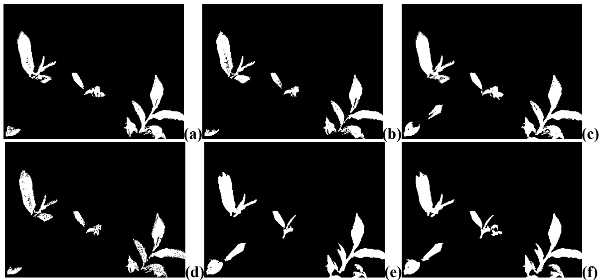
Fig. 4 Example results of image processing when the proposed indices were applied to the Figure 1(b), which was captured in the morning. (a) C_{yc} (b) C_{ym} (c) RI_{yc} (d) RI_{ym} (e) S channel. (f) U channel.
